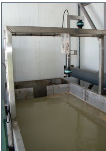
RECTANGULAR WEIR and DUET TRANSDUCER
