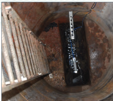
AREA X VELOCITY IN A CHANNEL USING SPEEDY and dBS6
