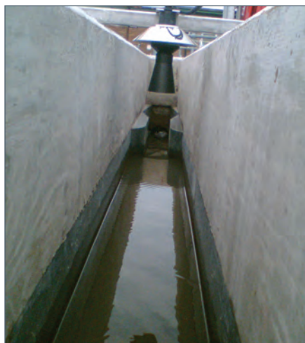
RECTANGULAR FLUME and dBMACH3
